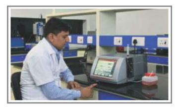
Auto Viscometer to test Viscosity & Density of Industrial & Automotive Lubricants
