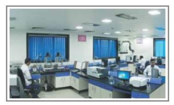
R & D Analytical Lab – II having FTIR for carbon type analysis, TNTS for Nitrogen and sulphur analysis, Foaming Tester, ICP for Elemental Analysis
